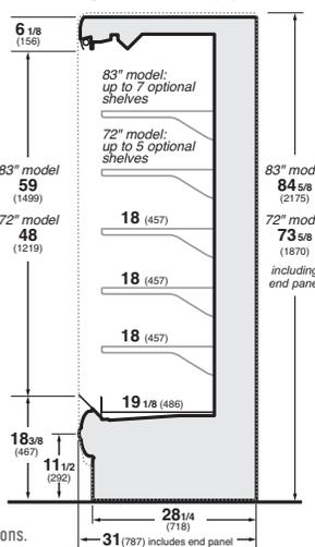
**RGD 24, 30 Remote and Self Contained plan view**
