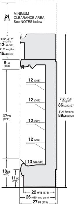
Maintain min. clearances as shown in dotted line area to facilitate air intake and discharge. Clean air circulation i.e. no air entrapment above unit so as to allow fresh air circulation
