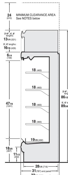
Maintain min. clearances as shown in dotted line area to facilitate air intake and discharge. Clean air circulation i.e. no air entrapment above unit so as to allow fresh air circulation
